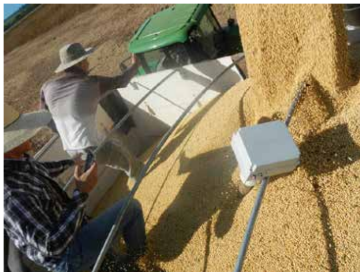
Grain probe installed in a truck to measure soybean conditions during transportation in Mato Grosso, Brazil. Credit: M.C. Danao
