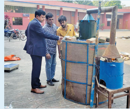
BAU researchers test the new Bangladesh-made blower on the BAU-STR dryer in December.
