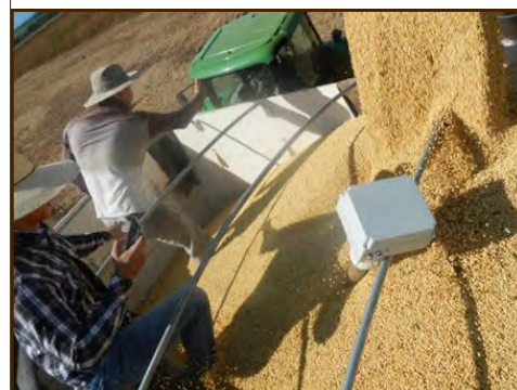
Grain probe installed in a truck to measure soybean conditions during transportation in Mato Grosso, Brazil. Credit: D.A. Williams
