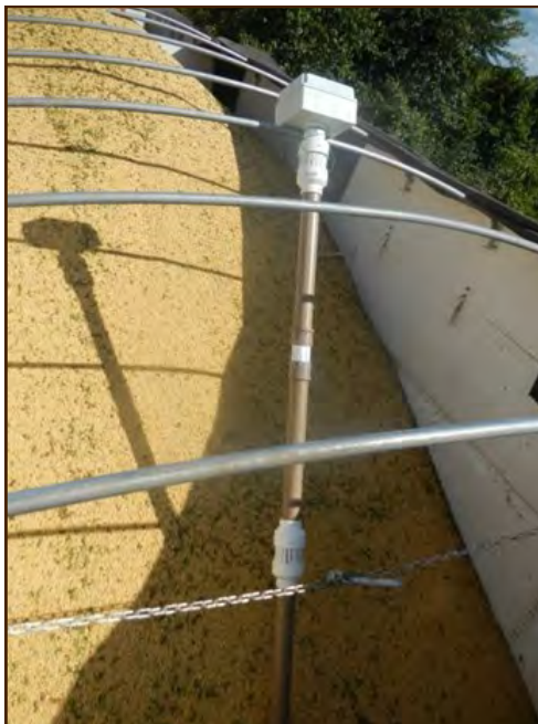
The probe Dr. Danao and her team designed to monitor grain condition during transportation. Credit: D.A. Williams
