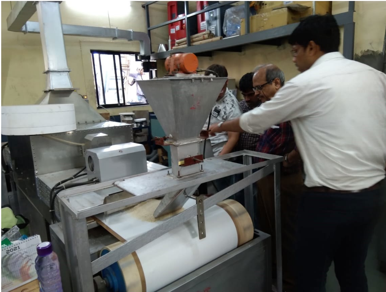
Treatment of Non-basmati rice in continuous microwave system
