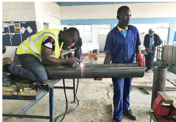
SIL trainers Imoro Donmuah (left) and Hakeem Abdul-Karim (right), from Ghana, show trainees in Ethiopia how to cut a pipe using a plasma cutter.
